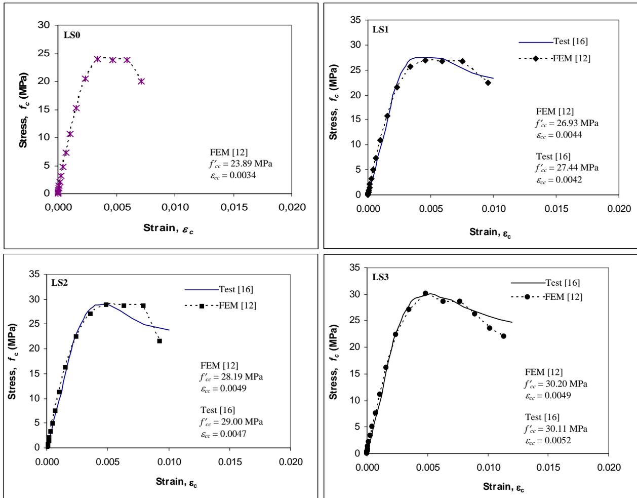
Figure 8. Stress-strain curves of column specimens LS0, LS1, LS2, and LS3
