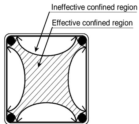
**Figur 1.** Effective and ineffective confined regions in a concrete core of a square column cross section produced by the arching action due to the existence of rectilinear confinement
