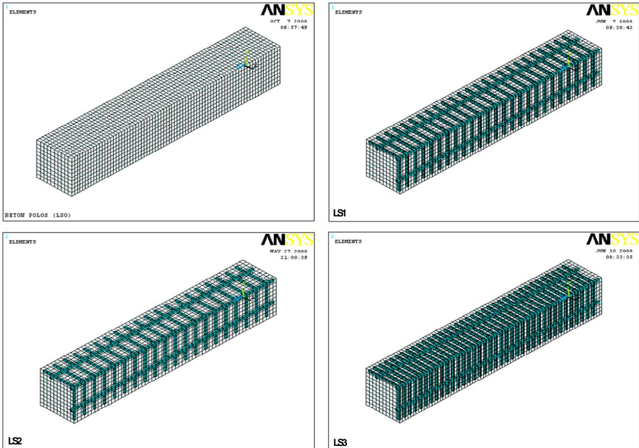
Figure 6. Element meshing of quarter column specimens LS0, LS1, LS2, and LS3
