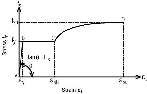
**Figure 5.** Stress-strain relationship for reinforcing steel proposed by Park and Paulay [19]
