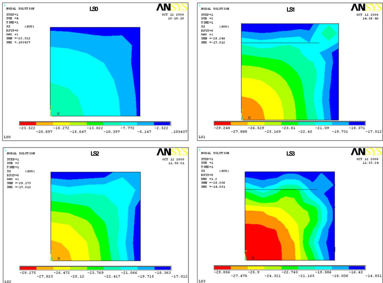
Figure 7. Axial stress distributions over the mid-height cross section of quarter column specimens LS0, LS1, LS2, and LS3
