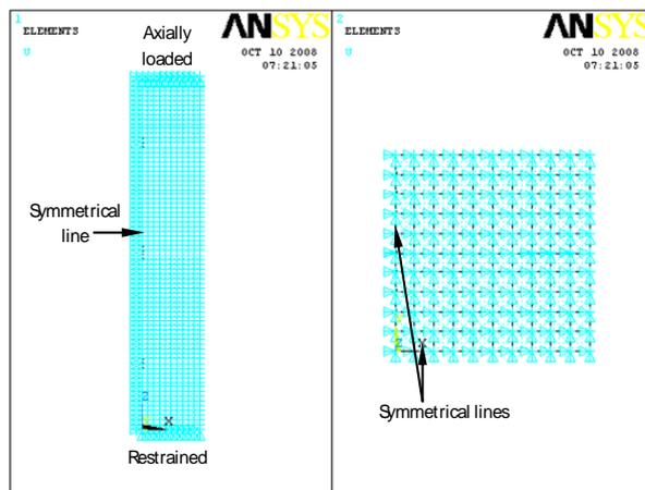
**Figure 2.** Boundary conditions of a symmetrical quarter of a column model: (a) elevation; (b) cross section
